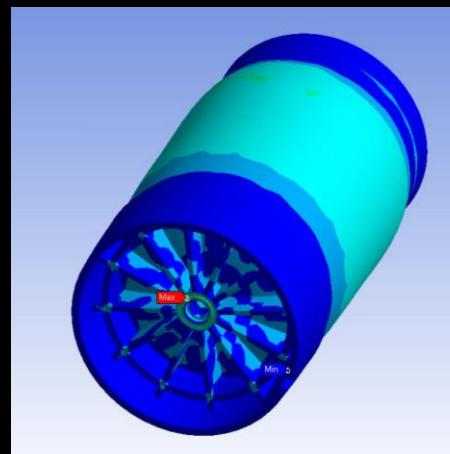
After the iterative process of testing various combinations using ANSYS DesignSpace software, the final design included a domed bottom surface with 12 radial ribs. The design lowered stress levels and wall thicknesses significantly, thereby cutting injection molding cycle time in half and lowering part cost by more than a third.
