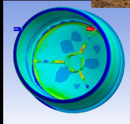
In spite of its 0.27-inch-thick bottom wall and three internal ribs, stress levels in the original water filter design exceeded the ABS material yield strength and showed up in red on the ribs, as displayed in this color-coded stress plot.
